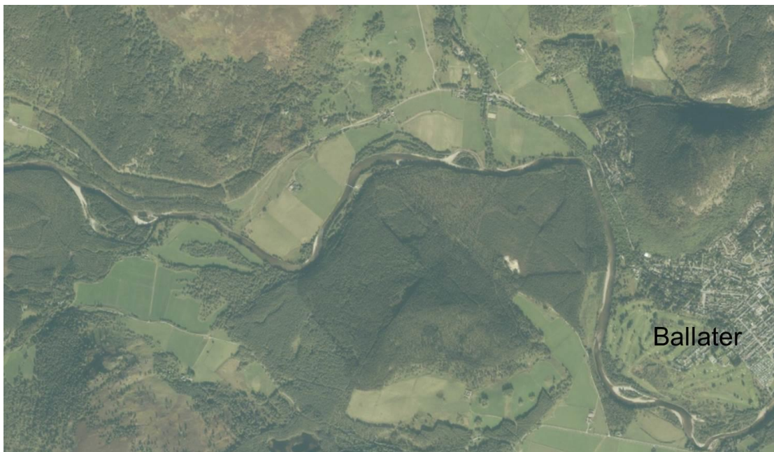
Figure 46: Recent aerial image of River Dee upstream from Ballater showing increase in sediment deposits in the channel.
